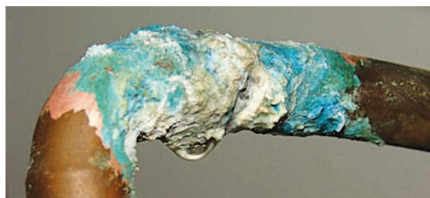
fig-18: Corrosion of copper
