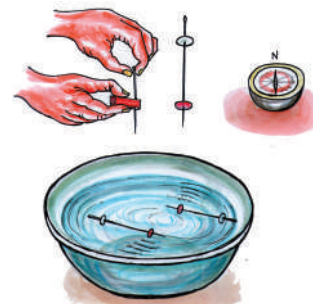
Fig-2: Making needle magnets and floating them in a bowl of water.
