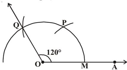
**Step-4:** With P as centre and without altering the radius (as in step 2) draw an arc which cuts the first arc at Q.
