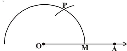
**Step-3:** With M as centre and without altering radius (as in step 2) draw an arc which cuts the first arc at P.
