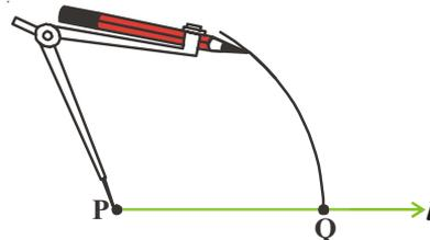
**Step-3:** Use the same compasses setting to draw an arc with P as centre, cutting  $l$  at Q.
