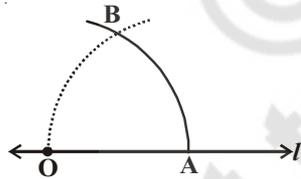
**Step-3:** With the pointer at  $A$  (as centre) and the same radius as in the step-2. Now draw an arc that passes through  $O$ .
