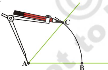
**Step-2:** Now place the compasses at A and draw an arc to cut the rays AC and AB.
