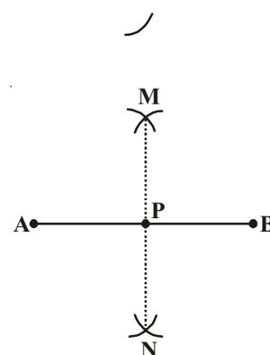
**Step-5:** Join the points  $M$  and  $N$ . Then, the line  $l$  is the required perpendicular bisector of the line  $AB$ . Line  $l$  intersects line  $AB$  at  $P$ .
