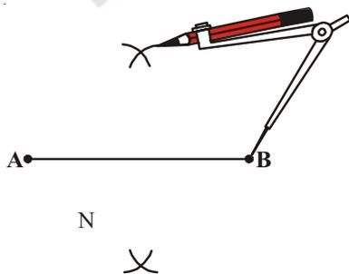
**Step-4:** With the same radius and  $B$  as centre draw two arcs above and below the line segment to cut the previous arcs. Name the intersecting points of arcs as  $M$  and  $N$ .
