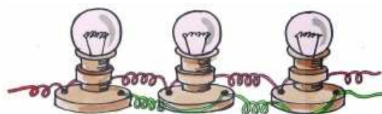
Fig. 13 - bulbs connected in parallel
