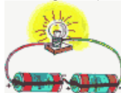
Fig. 9 - Connecting dry cells in series
